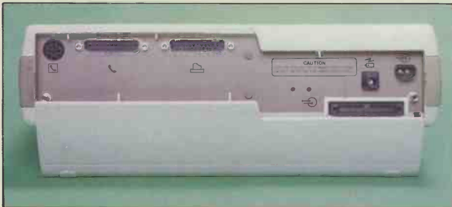
The One has two RS-232C ports for a modem and printer, plus an expansion socket.
